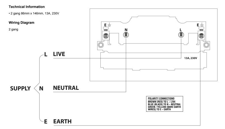
Safety - Suitable only for indoor installations Before starting any electrical work always switch off at the mains. If in any doubt consult a qualified electrician Ensure that the earth is connected otherwise it will be unsafe. Wire / Wiring colours in accordance with IEE Wiring Regulations
