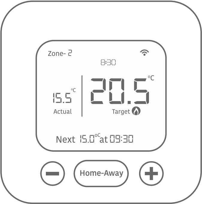
PTD after establishing communication with the receiver
