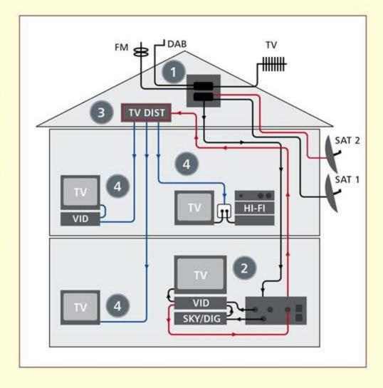
Method of installation of TV and FM aerial connection by using MK co-axial socket outlet and only one downlead.
