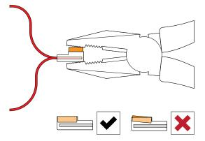
Do not strip wires. Insert both wires fully into UY2. Press down 'BUTTON' on UY2 using pliers.
