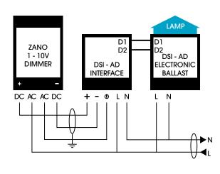
FOR LOW VOLTAGE CONTROL USE A 0.75MM<sup>2</sup> TWO CORE SCREENED CABLE, EARTH AT ONE END
