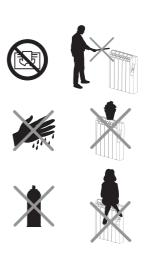
**WARNING!** In order to avoid overheating, don't cover the heater. Don't insert any kind of object in the air vents. Never use with wet hands. Don't place any containers with water, such as glasses, vases, etc. on the radiator. Don't use insecticides, paints or aerosols on the radiator. Don't sit on the radiator or place anything in front of it.
