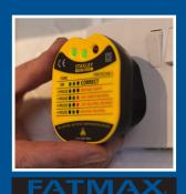
FatMax® Wall Plug Tester quickly checks the status of UK wall plugs. The LED lights clearly indicate a range of wiring conditions such as correct, missing earth and live earth reverse etc. This unit will not detect earth neutral reverse. Designed to Safety Standard EN 61010.
