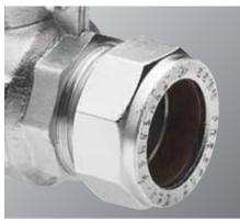
**1.** Select the correct size of tube for the job. Ensure that it is clean, in good condition and free from damage and imperfections. If the tube is oval or damaged, use a re-rounding tool. Copper tube should be of half-hard (R250) or hard (R290) temper. Annealed soft temper tube (R220) can be used.
