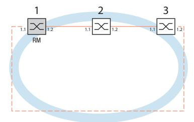
Figure 6: Example of MRP-Ring RM = Ring Manager —— main line - - - redundant line
