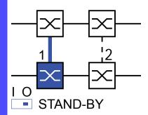
Figure 27: Two-Switch coupling
