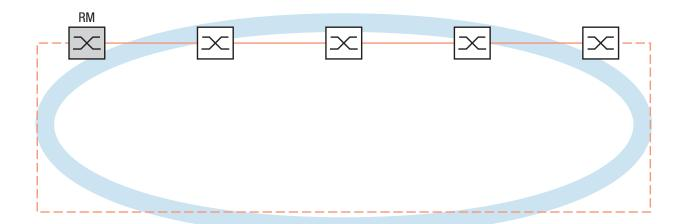
Figure 2: Redundant ring structure RM = Ring Manager —— main line - - - redundant line
