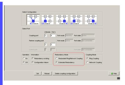
Figure 23: Selecting the redundancy mode
