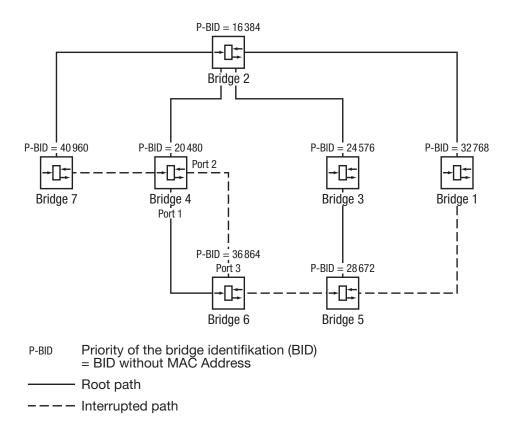
Figure 46: Example of tree structure manipulation
