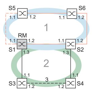
Figure 53: Application example for the combination of RSTP and MRP 1: MRP-Ring, 2: RSTP-Ring, 3: Redundant RSTP connection RM: Ring Manager
