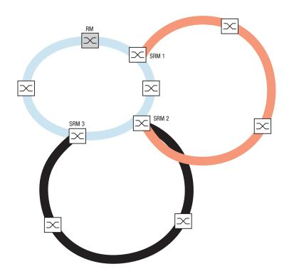
Figure 14: Special case: a Sub-Ring Manager manages 2 Sub-Rings (2 instances).
