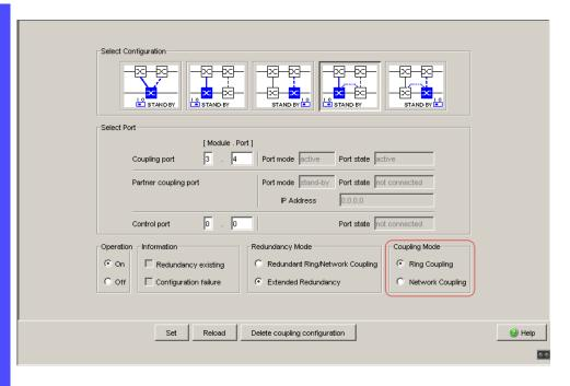
Figure 39: Selecting the coupling mode
