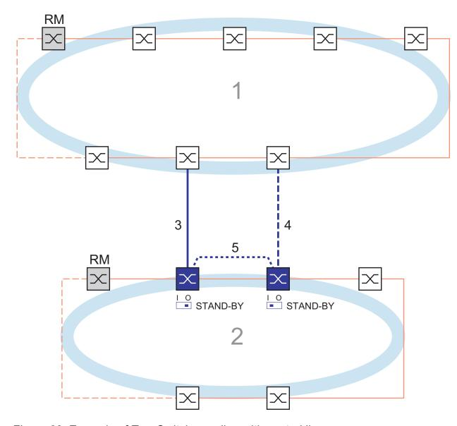
Figure 33: Example of Two-Switch coupling with control line
