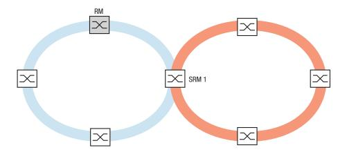
Figure 15: Special case: a Sub-Ring Manager manages both ends of a Sub-Ring at different ports (Single Sub-Ring Manger).
