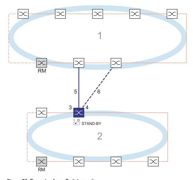
Figure 20: Example of one-Switch coupling
