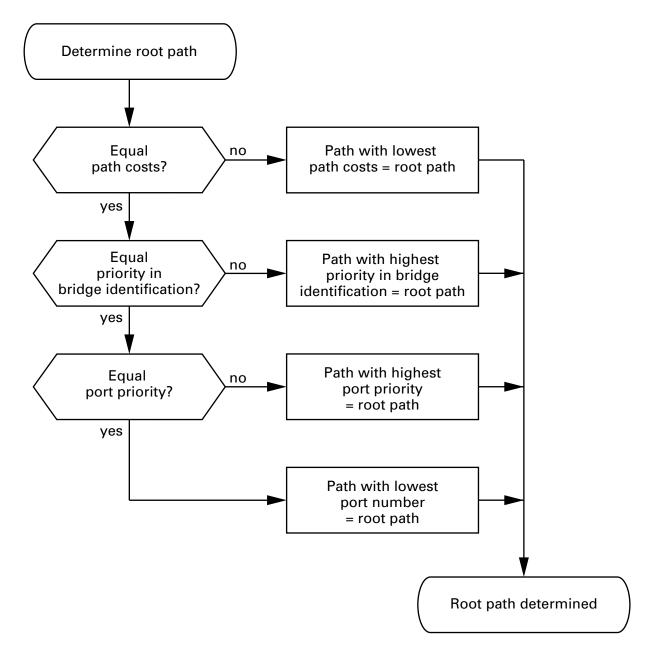
Figure 43: Flow diagram for specifying the root path
