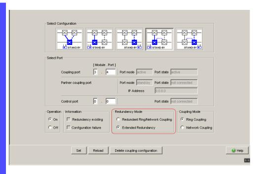
Figure 37: Selecting the redundancy mode
