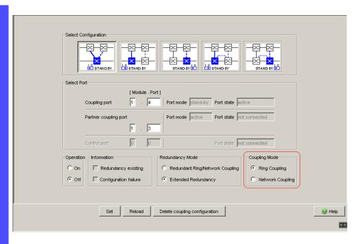
Figure 25: Selecting the coupling mode
