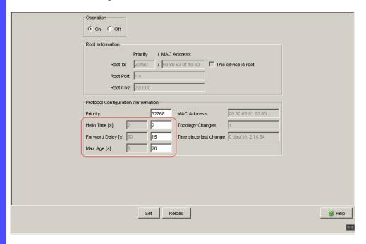
Figure 49: Assigning Hello Time, Forward Delay and Max. Age
