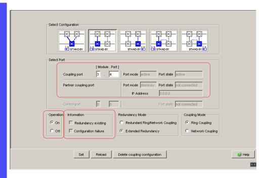
Figure 28: Selecting the port and enabling/disabling operation
