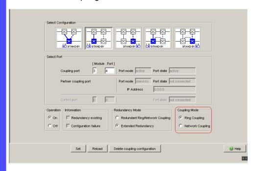
Figure 32: Selecting the coupling mode
