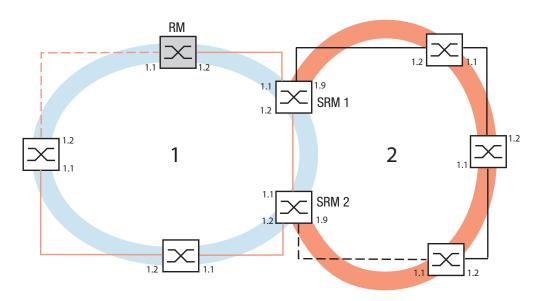
Figure 12: Example of a Sub-Ring structure
