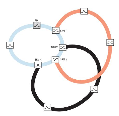
Figure 13: Example of an overlapping Sub-Ring structure
