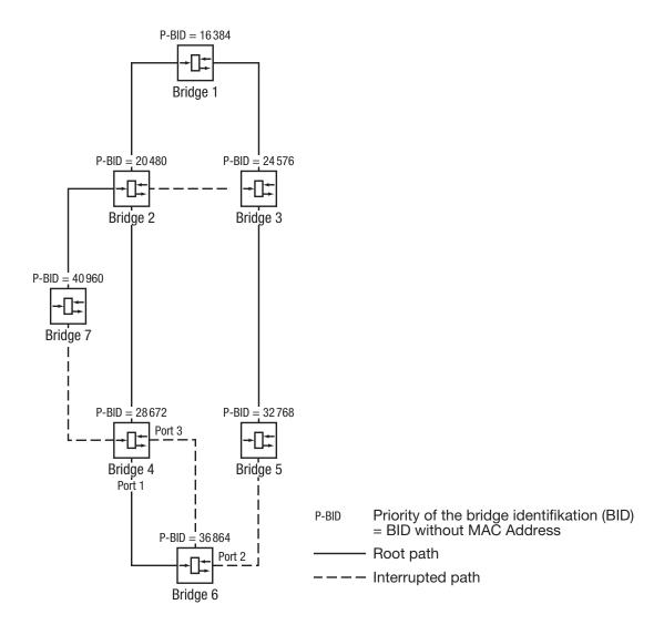
Figure 44: Example of root path determination
