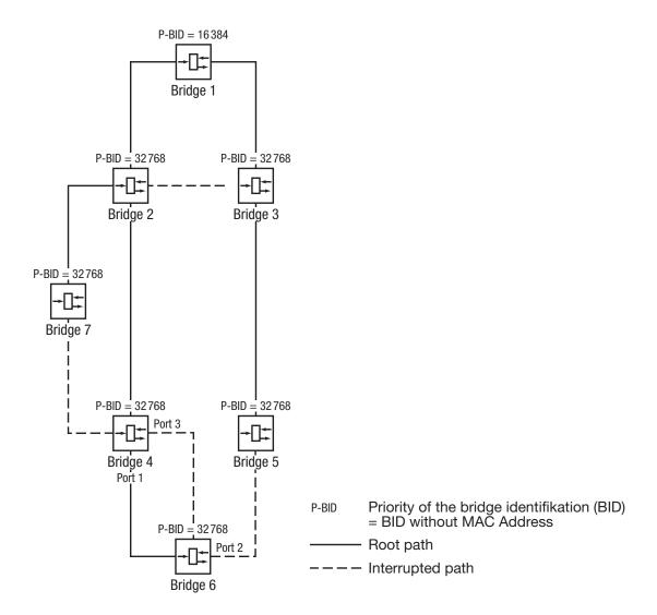
Figure 45: Example of root path manipulation
