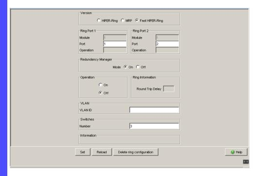
Figure 10: Ring Redundancy dialog (TCSESM-E)
