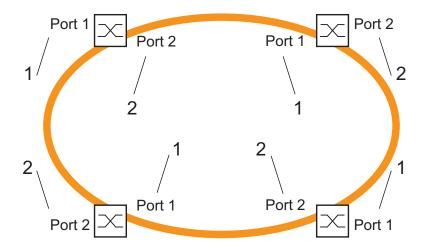
Figure 11: Example for a HIPER-Ring with straight cables 1 = Manual Cable Crossing disabled 2 = Manual Cable Crossing enabled
