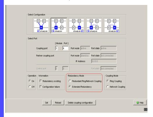
Figure 30: Selecting the redundancy mode
