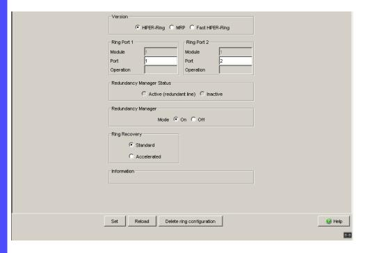
Figure 5: Ring Redundancy dialog (TCSESM-E)
