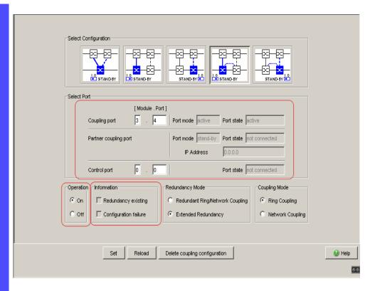
Figure 35: Selecting the port and enabling/disabling operation
