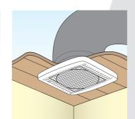
**Ceiling Mounting** Hole Diameter: 150mm
