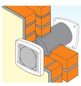
Wall Mounting using Wall Mounting Kit Hole Diameter: 165mm Ducting Size: 150mm
