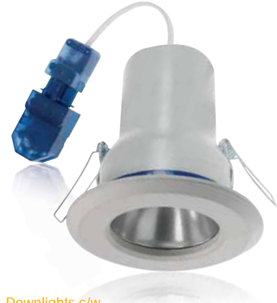
230V Cast Fixed 118mm Dia. Downlights c/w Flow™ Connector & Moisture Seal
