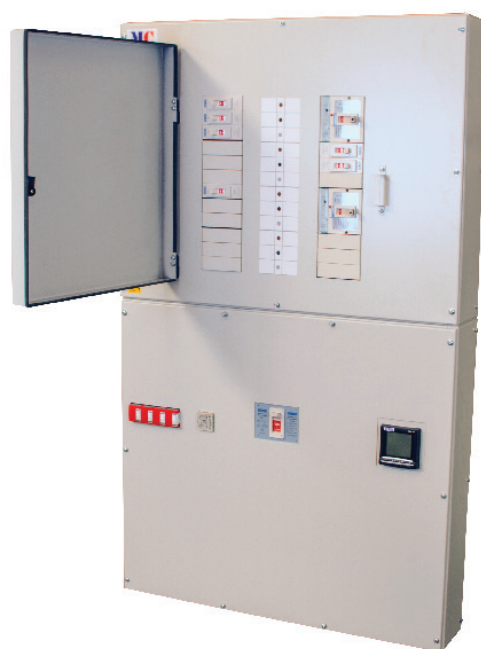
MCP88/I630 Options shown - MCP630, MCPDMM630T and MCPT12/TNSIF Outgoing switchgear supplied separately
