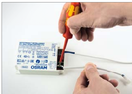
Step 2: Connect cables to DALI dim driver
