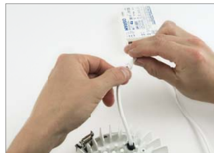
Step 3: Quick connection to luminaire
