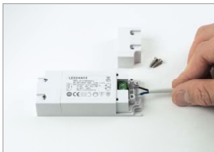
Step 1: Unscrew cover and connector cables
