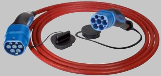
Charging cable (mode 3), 32A with charging plugs and charging connector 1P+N+PE as well as PP + CP
