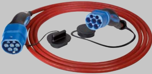
Charging cable (mode 3), 20A with charging plugs and charging connector 1P+N+PE as well as PP + CP
