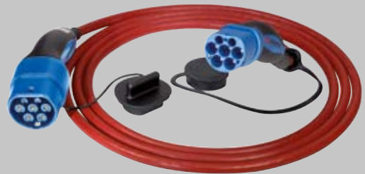
Charging cable (mode 3), 32A with charging plugs and charging connector 3P+N+PE as well as PP + CP
