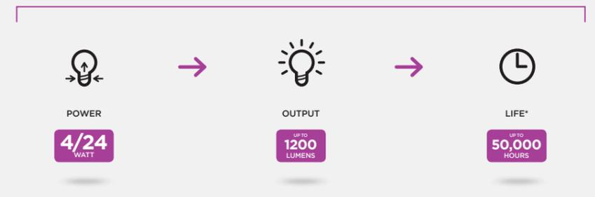
\* We test our lamps to both L70 and L90 standards. Figure shown is for L70. Operating temperature -30°C to +40°C
