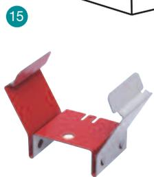
15 Multi-purpose clip allows separation of power and data cables - ensuring a 50mm distance between cables or can accommodate the dividing fillet.
