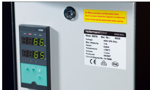
Professional type plate on a heating unit.
