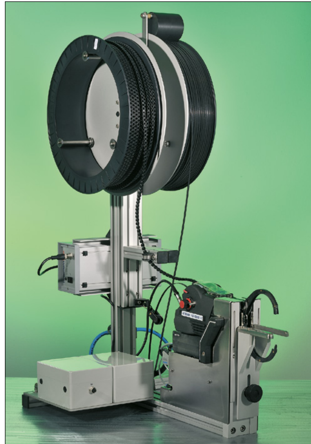
For the stationary installation – the bench mount kit.
