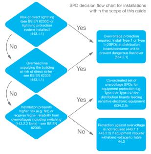
**Note:** For larger installations beyond the scope of this guide, a risk assessment method used to evaluate the need for SPDs is given in Section 443 of BS 7671:2008(2011)
