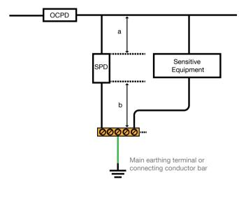
OCPD = overcurrent protection device SPD = surge protection device Should the distance between the SPD and the sensitive equipment to be protected be greater than 10m, oscillations could lead to higher voltage values appearing at the equipment. Consideration should be given to additional coordinated surge protection devices closer to the equipment. Again manufacturer's instructions should be followed
