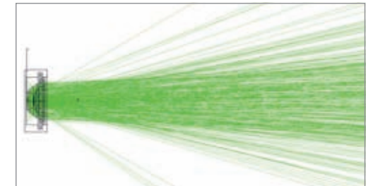
GEWISS SOLUTION POWER LED + TIR COLLIMATOR + SECONDARY LENS
