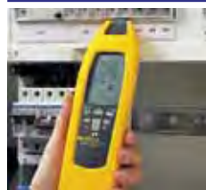
Location of fuses/breakers and assignment to circuits
