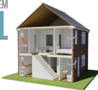
Intermittent extract fans with background ventilators
