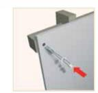
Mark out and drill fixing holes. Insert toggle
