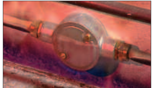
Appropriately jointed Firetuf cables continue to provide circuit integrity up to the full BS 5839 rating.
