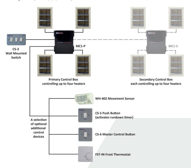
For larger installations up to eleven secondary control boxes can be connected in a control daisy chain with each controlling up to four additional heaters.
