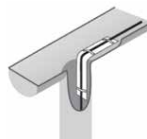
GP-S spacer protecting GP-18 cable from a sharp edge
