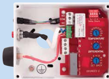
HC-ST2 Internal View Note adjustment knobs for both comfort and set-back settings
