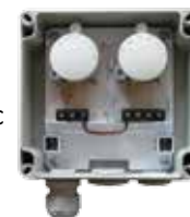
GP-T with cover removed showing set-point adjustment knobs
