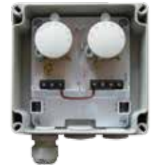
GP-T with cover removed showing set-point adjustment knobs
