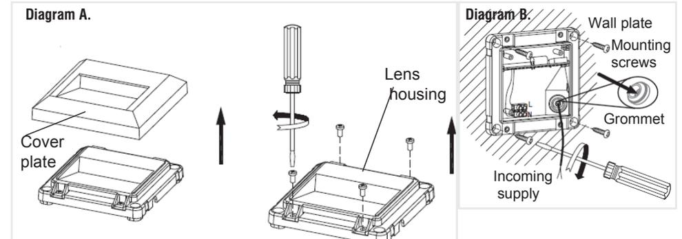
4 retaining screws on the sides of the unit. Unscrew these to remove the lens housing.
