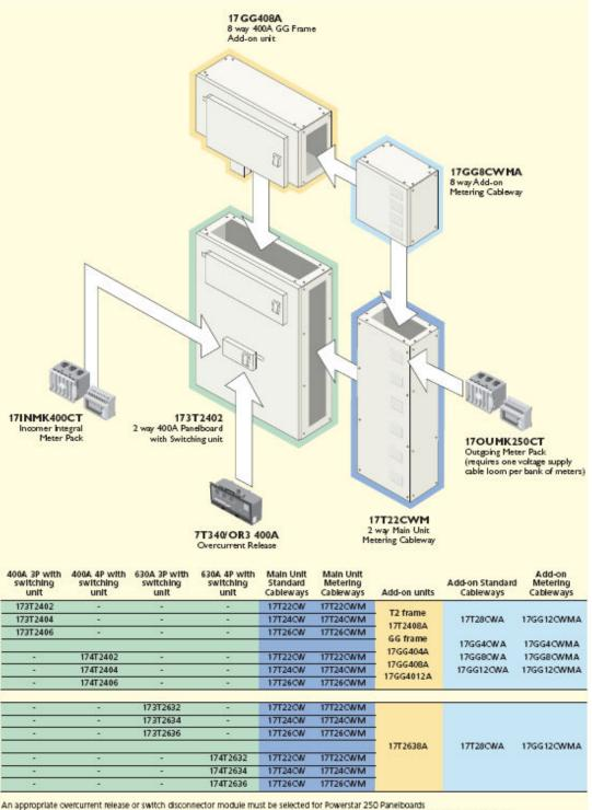
Each bank of outgoing main or add on unit meter packs to must be installed in conjunction with a voltage supply cable loom (170UMKCL) Product list numbers and descriptions can be found within the body of the catalogue
