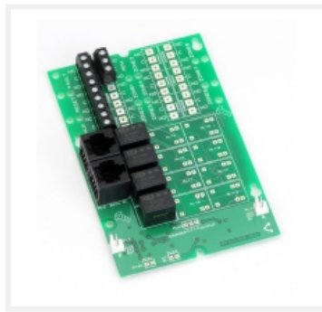
CFP Relay Output Card (Reset, Fault, Aux. &...
