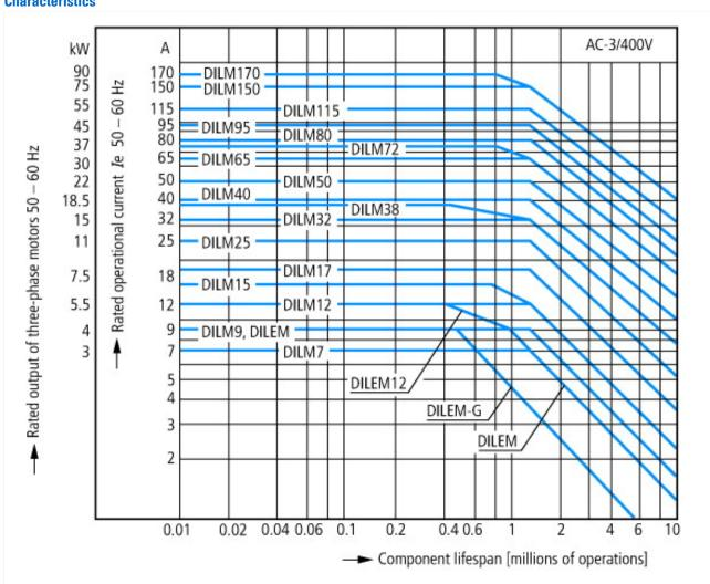
Squirrel-cage motor Operating characteristics Starting:from rest Stopping:after attaining full running speed Electrical characteristics Make: up to 6 x rated motor current Break: up to 1 x rated motor current Utilization category 100 % AC-3 Typical applications Compressors Lifts Mixers Pumps Escalators Agitators Fans Conveyor belts Centrifuges Hinged flaps Bucket-elevators
