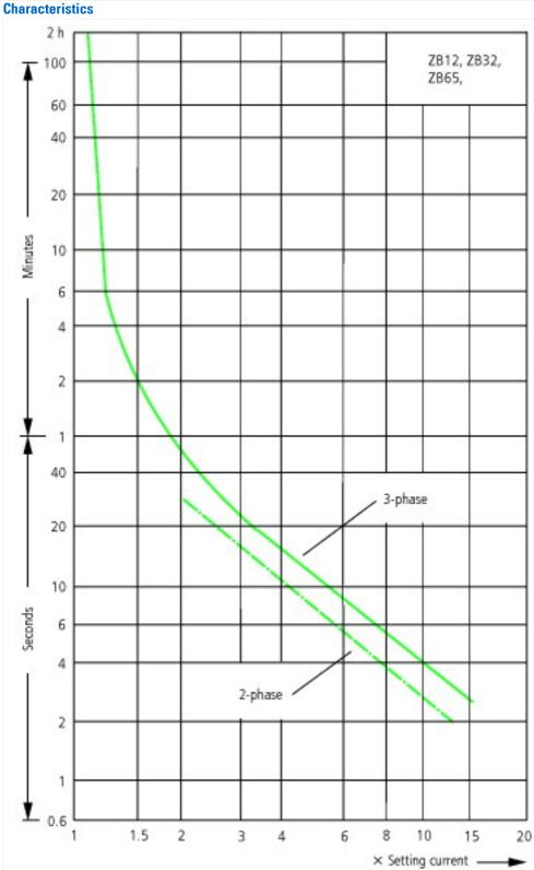
These tripping characteristics are mean values of the spread at 20 °C ambient temperature in a cold state. Tripping time depends on response current. On devices at operating temperature the tripping time of the overload relay drops to approx. 25 % of the read value. Specific characteristics for each individual setting range can be found in the manual.
