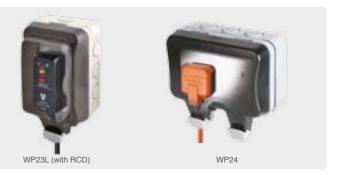
• IP66 Rated with plug in use, cover sealed RCD sockets manufactured to BS 7288 30 milli-amp trip current, 40 milli-second trip speed
