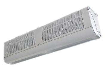
These units are 1305 mm 9 or 12 kW air curtain heaters designed for mounting above entrances. The discharge width of the air curtain is one metre. It is supplied complete with a remote mounting control box. These Screen-Zones may also be used as a space heater for commercial and industrial interiors. The appliance may be supported/mounted in a variety of ways.
