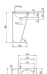
Single washbasin with rear upstand, single tap hole, 32mm BSP waste fitting and complete with three sided pedestal manufactured from stainless steel. Fittings include swan-neck spout and foot-operated timed control push valve for use with a pre-mixed water supply. Screws and dowels included.
