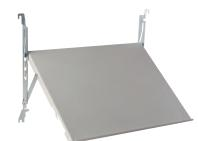
**Description:** Mounted directly to the door frame it provides a solid surface for documents, computer or measuring devices. The desk can be easily folded and locked within the door frame space. An automatic safety positioning system locks the desk at angles of 55°, 70° and 90°. The DDK800 can also be mounted on a 1000mm wide door, by the use of the DCP1002 accessory.
