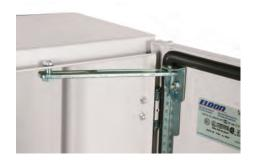
**Description:** Door stop for height 300mm enclosures and above. To secure the door in an open position allowing a 90° or 110° opening. Mounted directly to the door profile studs. Machining is required.
