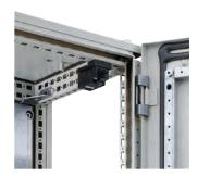
Description: Activates any electrical device (lighting, coolers, etc). Can be fitted after installing the enclosure thereby keeping the door opening free. Fixed (without screws) on the inside hole pattern of the enclosure's frame. Cable entry M 20.
