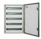
Description: Used for easy mounting of DIN-rail components with a maximum height of 68mm. Distance between rows 125mm. If required, the standard enclosure door can be replaced with a glazed door. Usable depth between front cover and external door: 35mm. Adjustable depth position with AMG accessory. In stainless steel enclosure machining is required. Material: DIN-rails PP0735 made of 1.20mm galvanized steel, vertical profiles 1.5mm mild steel, and front cover 1.5mm mild steel.
