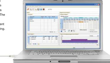
The windows software gives complete control of your heating system. Once programmed, the information will be sent to the USB transmitter which can then be disconnected and will continue to give the programming signals to the heating system. The RF control system is an option, but there are also other ways of setting up your Digi-Line heating system.
