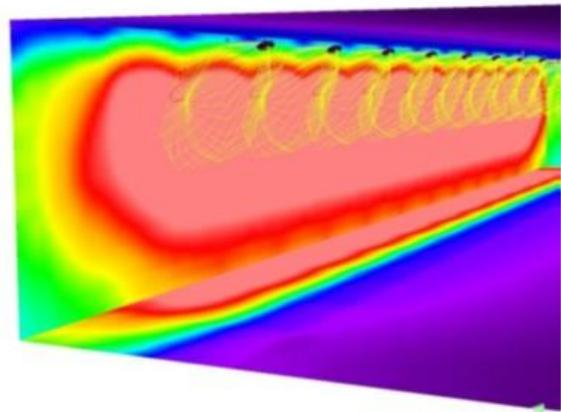
With this new design of optics, the position of the Highspot LED can be brought in tight to the surface to be lit, therefore reducing any glare experienced by customers (*see image below*).
