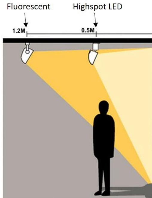
The reduced mounting distance also makes the Highspot LED retail spotlight suitable for use in narrow shop windows. The product incorporates innovative thermal cooling, so no cooling fan is required despite its 4000lm output and compact design.
